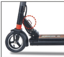
Step 5: Pull out the red lever, and fold the scooter stem at the same time
