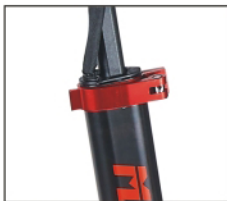
Step 3: unscrew the nut and loose the buckle
