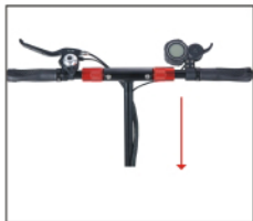
Step 4: Pull downward the T handle bar
